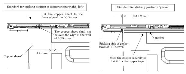
Figure 4-50 Sticking the copper sheets and gasket
